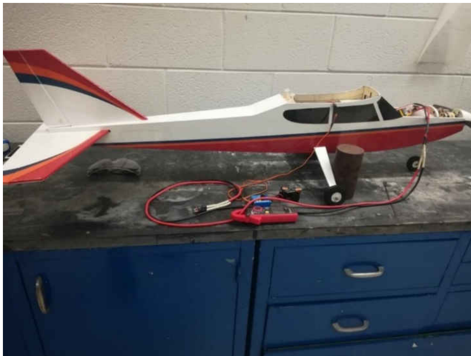
Figure 4.8 AVISTAR RC plane fixed on the lab table for current discharge experiment
