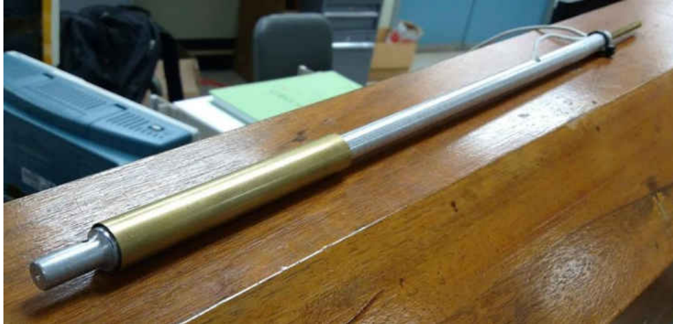
Figure 12: Sting with MS-100, brass sleeve, threaded rod, and standoff installed.
