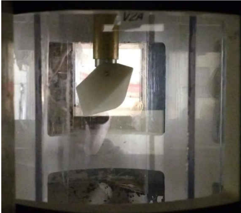
Figure 29: Top view of the 45° sting supported model (Flow is directed upwards in picture).
