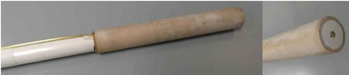
Figure 13: Second dummy sting with cavity pressure tap.
