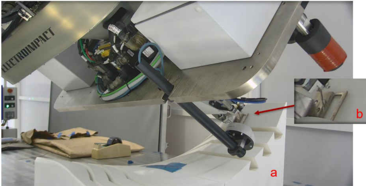
Figure 6 Presser Foot Collision: (a) 3D Printed Surface to hold Fabric, (b) Presser foot collision with surface without fabric
