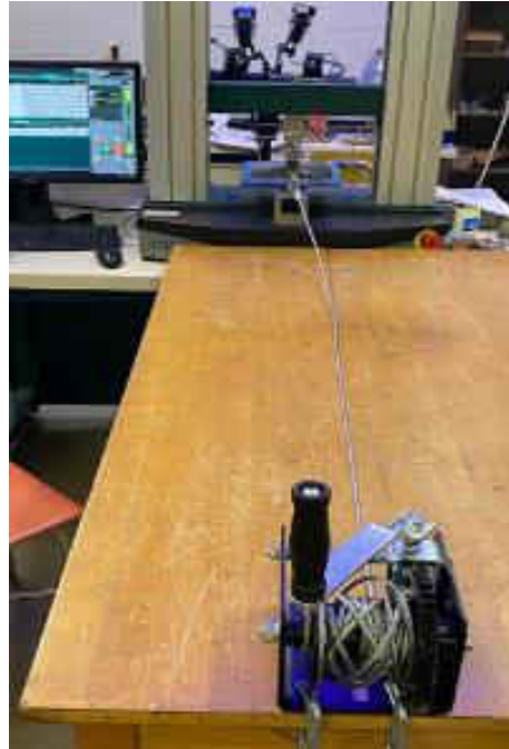
Figure 72 Winch and DIC Setup
