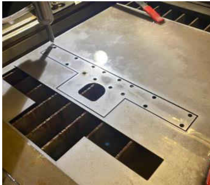
Figure 24 Wrinkling Fixture Water Cutting Process
