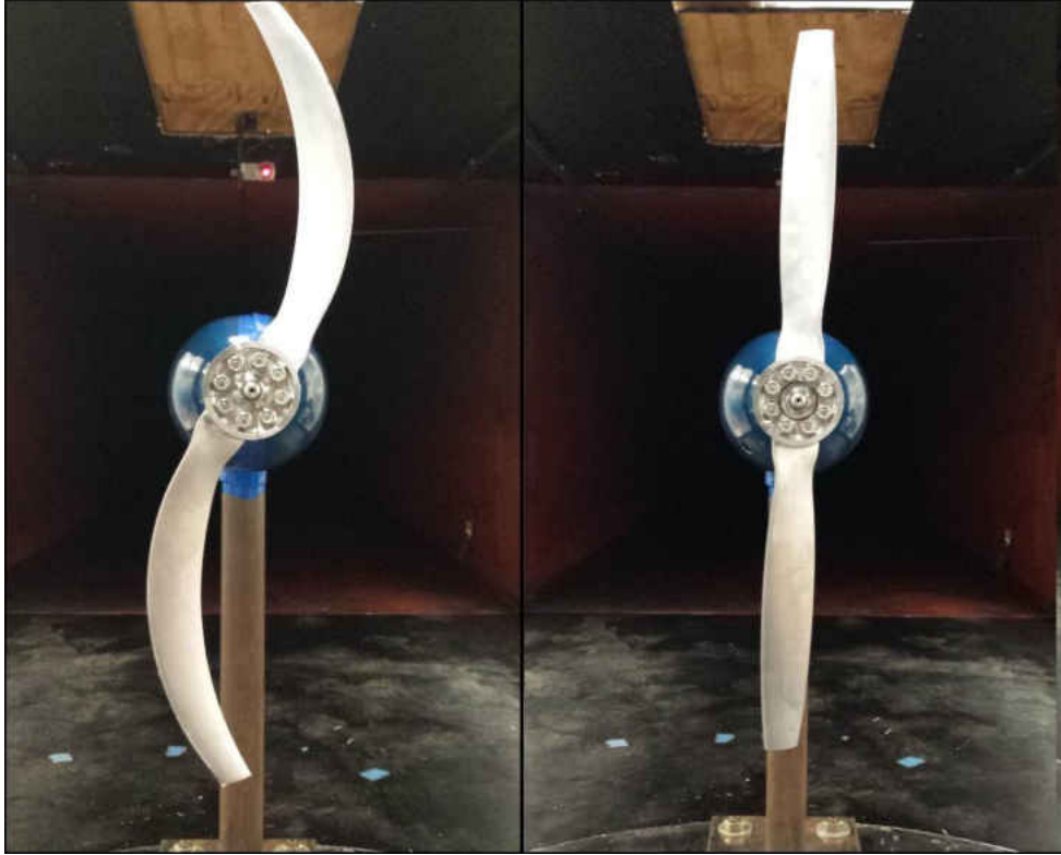
Figure 62: Swept-35 (left) and straight (right) inside ODU's wind tunnel.
