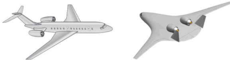
Figure 19: Conventional tube-and-wing and unconventional Hybrid Wing Body aircraft designs. [30]
