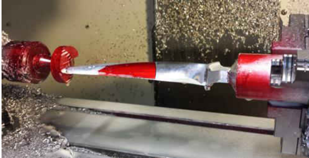
Figure 36: One of the swept-15 propellers used to test for production errors.
