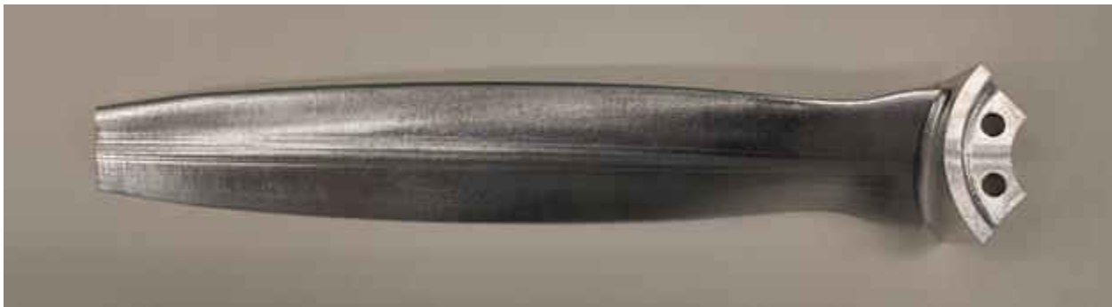
Figure 34: The conventional, straight propeller after milling with the 4DOF method.
