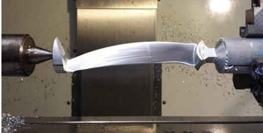
Figure 35: The swept-15 propeller held in with the tail stock and rotary table for the 4DOF milling method.
