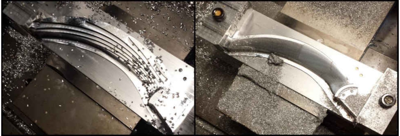
Figure 32a & 32b: 32a presents the 1st rough cut of milling with the 3DOF method and 32b presents the 2nd finer cut.
