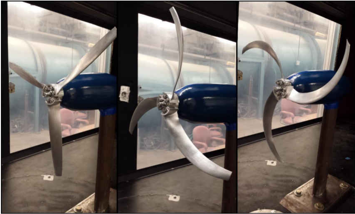
Figure 66: The three different designs tested in ODU's wind tunnel for the three-blade configuration.
