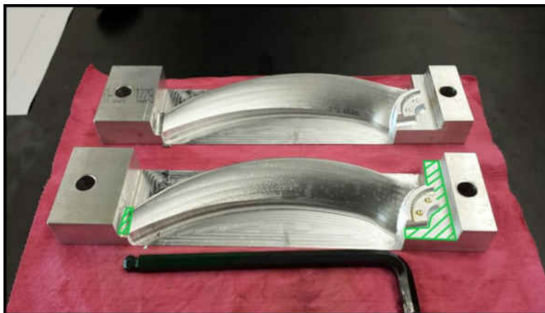
Figure 33: Two swept-35 propellers made in the 3DOF miller with the top side milled away. The highlighted portions would be trimmed after the underside was milled.
