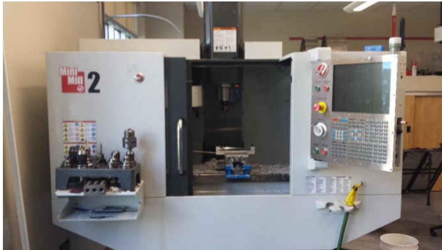
Figure 31: The Super Mini Mill 2. This CNC machine was used to mill all 16 propellers.
