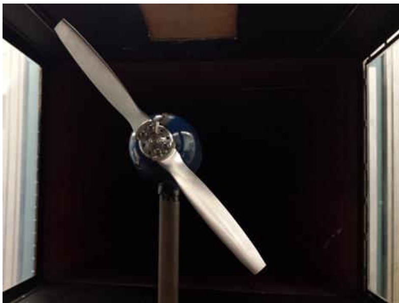
Figure 4 – 16 in straight blade propeller inside ODU LSWT
