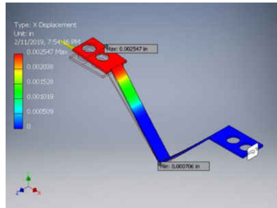
Figure 20- FEA on copper spring in the X-Displacement
