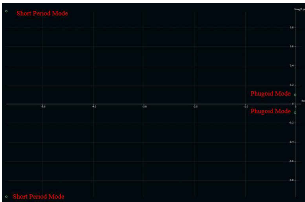
Figure 72-Root locus plot of longitudinal modes for EdgeTRA
