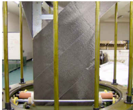
Figure 3. An automated lamination machine created by the Mitsuya Company. [7]
