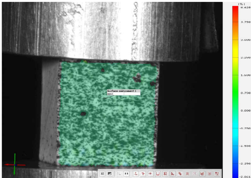
Figure 41 Strain measurements are recorded by the DIC system at 15th sec for 90-degree off-axis loading.
