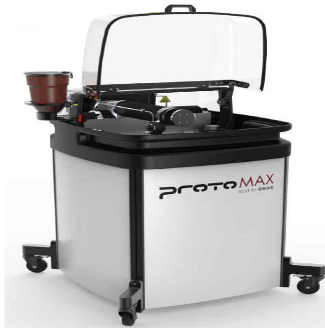
Figure 6 Represents the water jet cutting system
