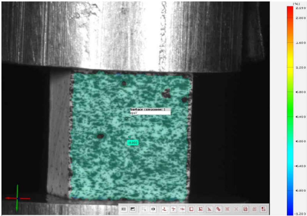
Figure 42 Initial surface component of the y-component in the applied direction
