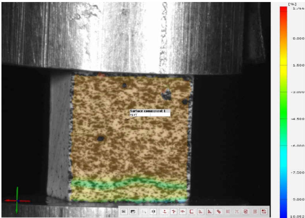
Figure 43 Strain measurements recorded by DIC system at 15 th sec of y-component
