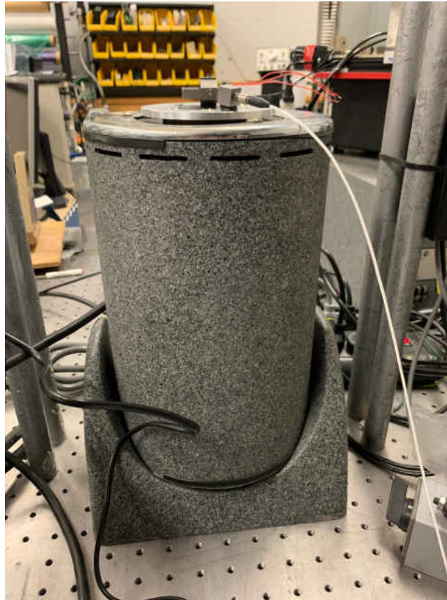
Fig. 16: Dynamic experiment setup of Flextensional Piezoelectric Energy Harvester
