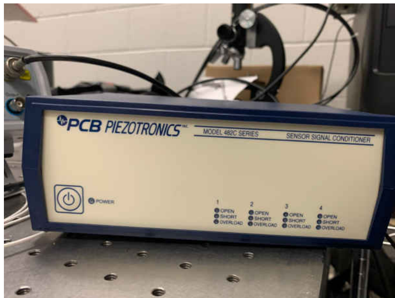
Fig. 20: PCB 482C Series 4-Channel Signal Conditioner
