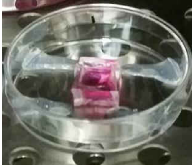
Figure 2. Cells are plated and confined within a Polydimethylsiloxane (PDMS) well placed in the middle of an electrotaxis chamber.
