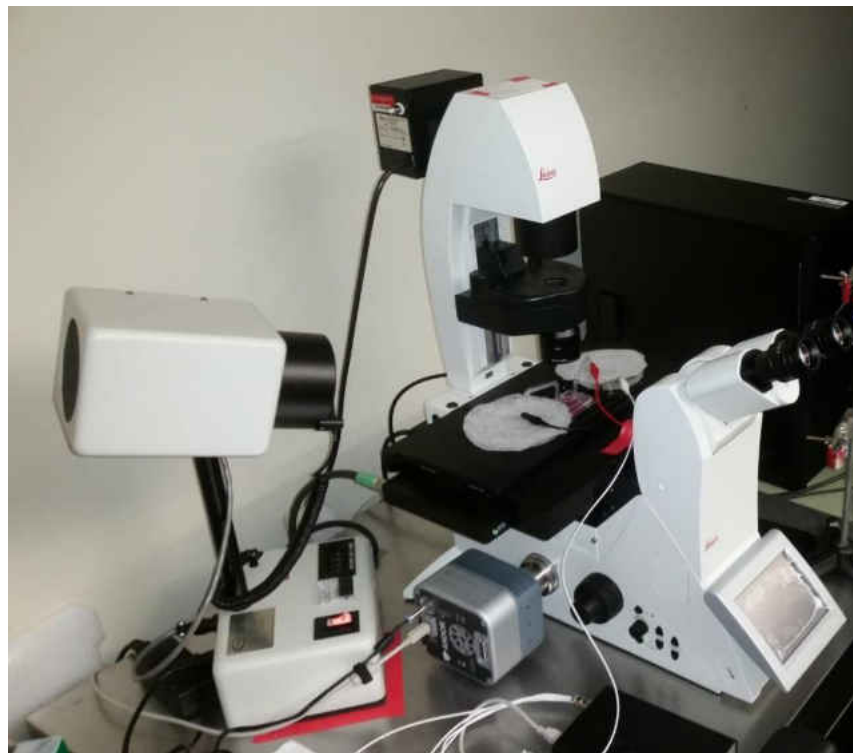
Figure 4. Experimental setup for imaging monolayers during electrotaxis
