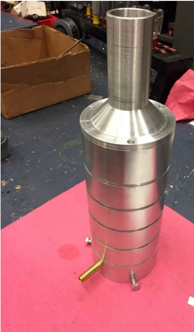
Figure 3.12. Inertial cascade impactor after leaving the machine shop.
