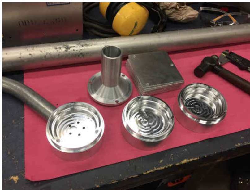
Figure 3.11. Several parts manufactured on CNC milling machine
