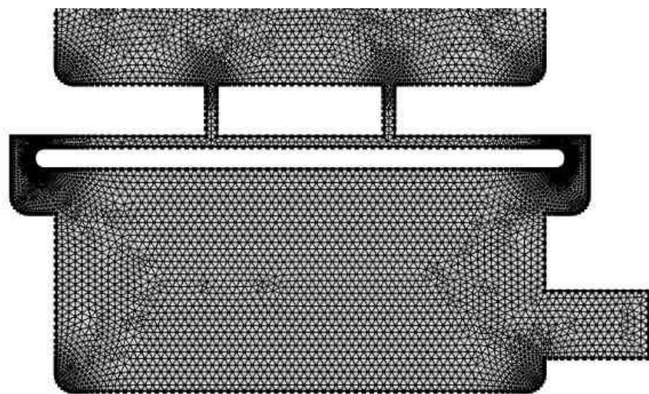
Figure 2.8. Stage 5 Mesh generated by COMSOL.
