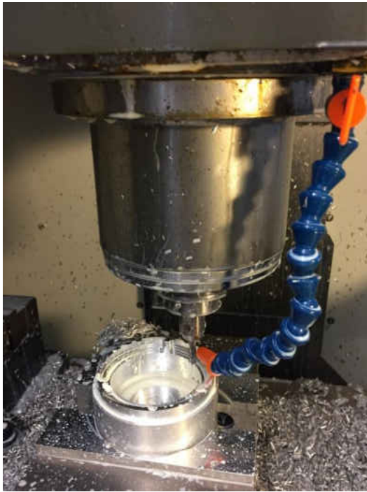
Figure 3.9. Manufacturing base on CNC milling machine
