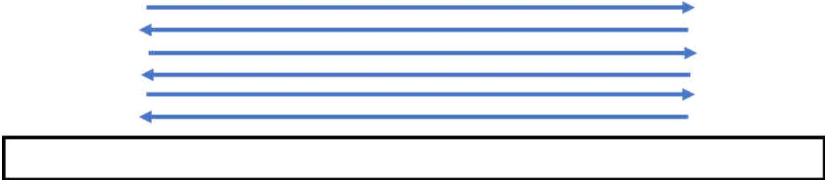
Figure 5. Illustration of welding direction for WAAM wall
