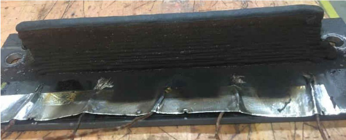
Figure 6. The AM part after completion with thermocouples attached (Done at Clarkson University)
