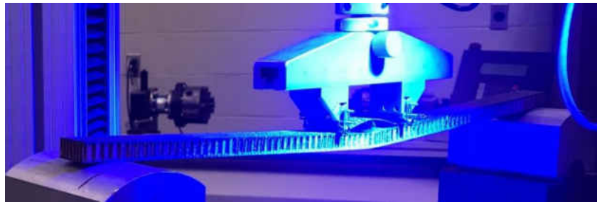
Figure 36: Failure of 8 ply unidirectional delaminated sample
