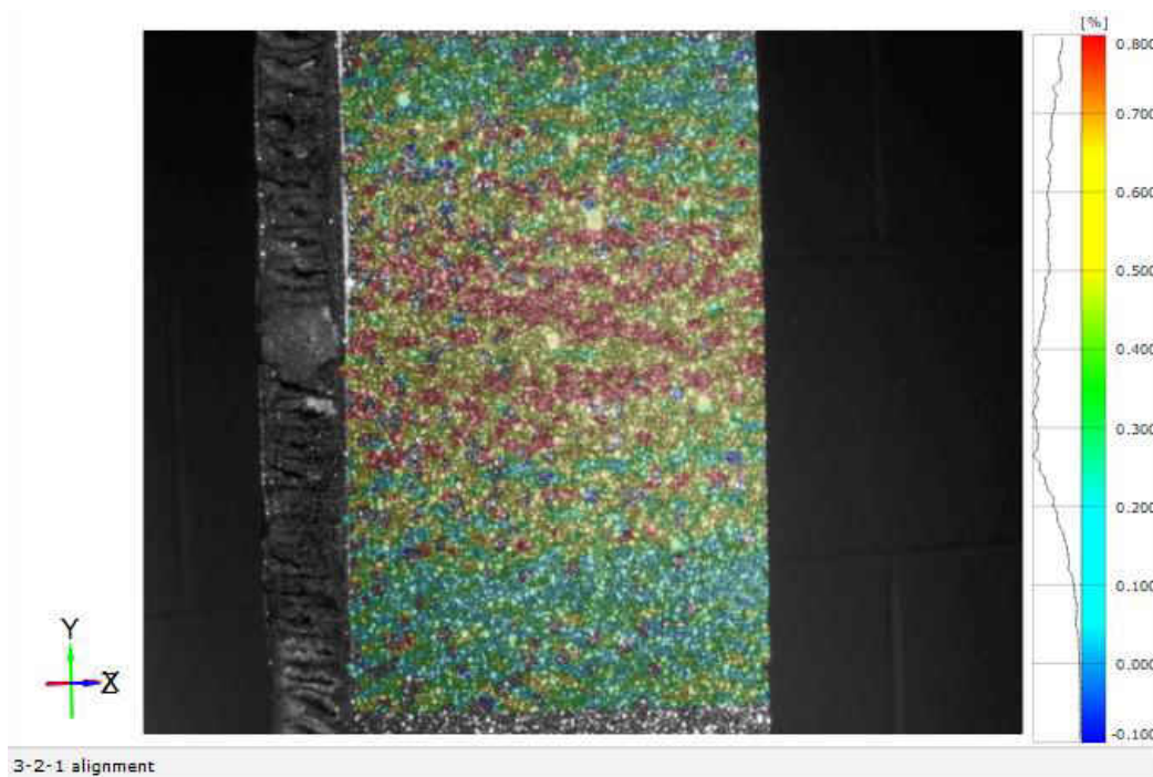
Figure 91: DIC strain image of a DLJ sample with a 1/2" delamination and TTR before failure
