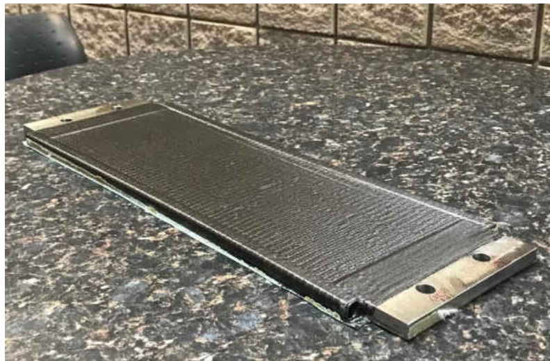
Figure 64: Successful curing of a panel in the autoclave
