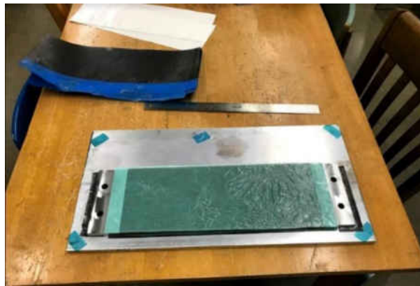
Figure 55: Fabrication of a double lap joint panel
