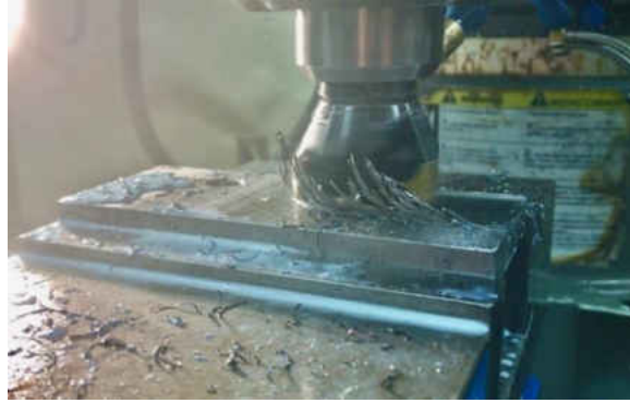
Figure 54: Machining of end adaptor plate in ODU's machine shop
