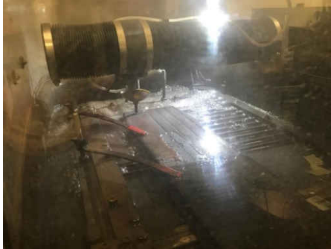
Figure 7: Waterjet cutting of a panel
