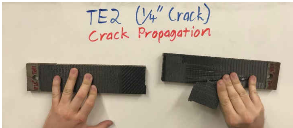
Figure 76: Crack propagation failure of a double lap joint 1/4" defect sample (front)
