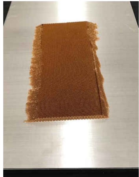
Figure 62: Tapered cutting attempt of honeycomb core
