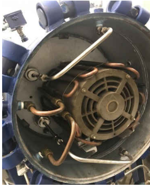
Figure 68: Repair of Autoclave
