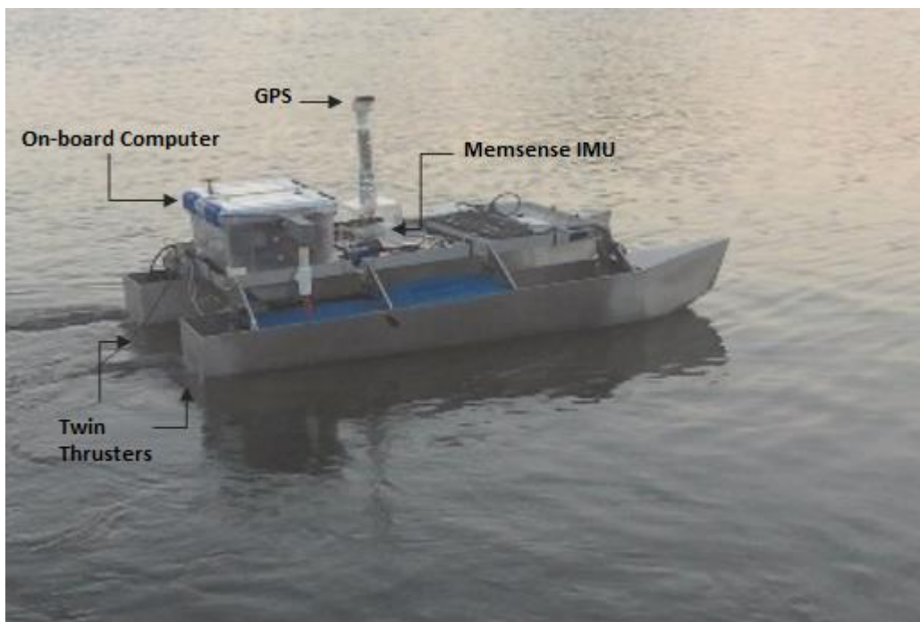
Figure 6.3 ODU-ASV while cruising for the purpose of data acquisition for OKID identification.
