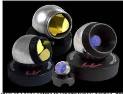
Figure 29: Cat Eye and SMR Reflectors [18]
