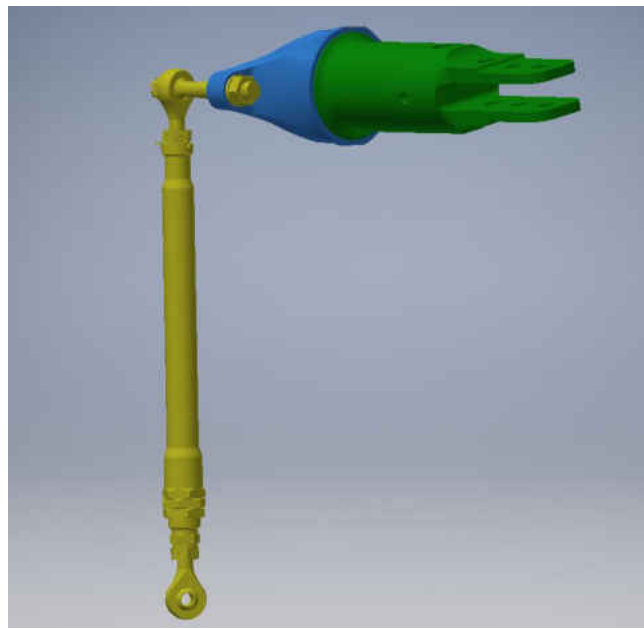
Figure 2: Pitch Link connected to pitch horn and blade grip
