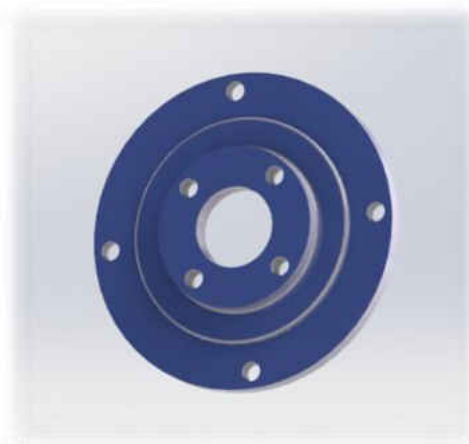
Fig. 3. 4 Part 2: Attachment for Part 1 that attaches to the Sawyer arm
