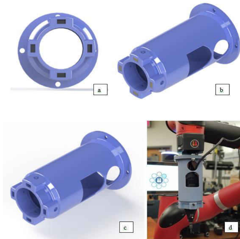
Fig. 3. 3 Attachment for Dremel Drill to be attached, a) Bottom view of Part 1, b) Side view of Part 1 with Steel blocks (c) Side view of Part 1 without Steel blocks inserted d) Drill attached to the Sawyer Robot Arm
