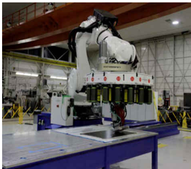
Figure 12: AFP Lay up example
