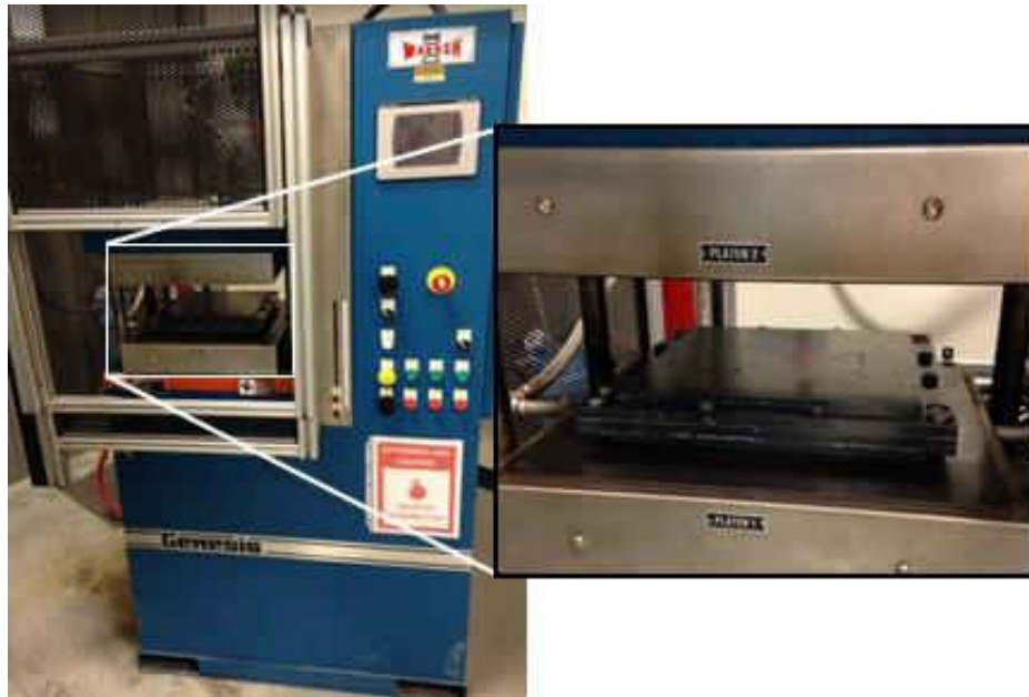
Fig. 7: Heated press used for making prepreg platelet molded composites.
