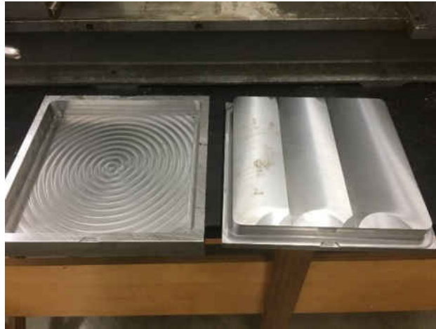
Fig. 5: Mold used to make 254 mm plate.
