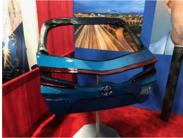
Fig. 3: Rear door of the new Toyota Prius, made of prepreg platelet molded composites.
