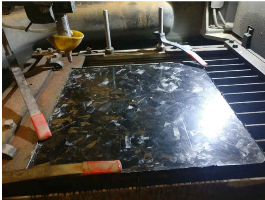
Fig. 8: Panel of 25.4 mm platelet material in the waterjet. The panel is ready to be cut into 9 specimens for testing.
