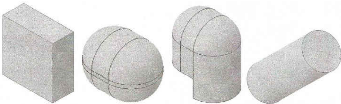
Figure 4: Third Solid Modeling Attempt using Autodesk Inventor (from left to right: computational domain / brain, CSF, skull, and impactor)
