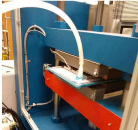
Figure 8: Vacuum bagging setup with heated platens.
