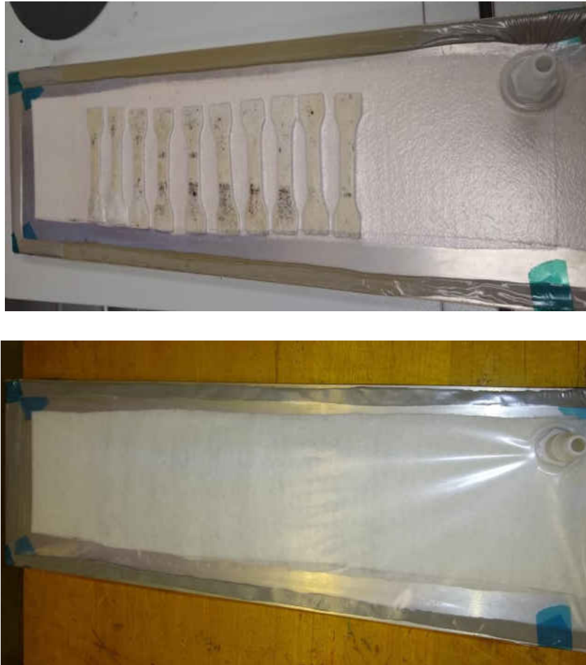
Figure 10: Vacuum bagging setup-before and after heat treatment
