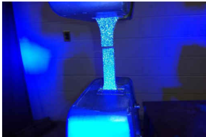
Figure 12: Tensile testing setup with DIC
