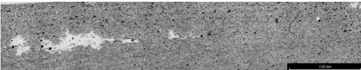
Figure 34: Micrograph of polished cross section of samples annealed at 170 with 0-degree print orientation
