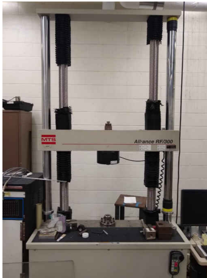
Figure 11: MTS machine used for tensile testing
