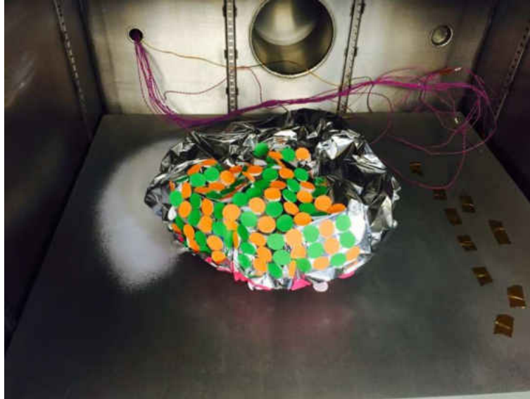
Figure 55. Ruptured Benzoic Acid Test Article Showing White Benzoic Acid Residue
