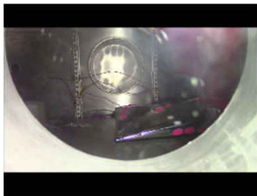
Figure 42. Air Inflatable (12 torr)
