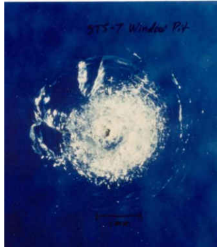
Figure 8. STS-7 Windshield Damage from Orbital Debris 8
