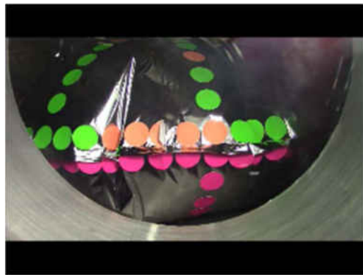
Figure 47. Air Inflatable (0.5 torr)
