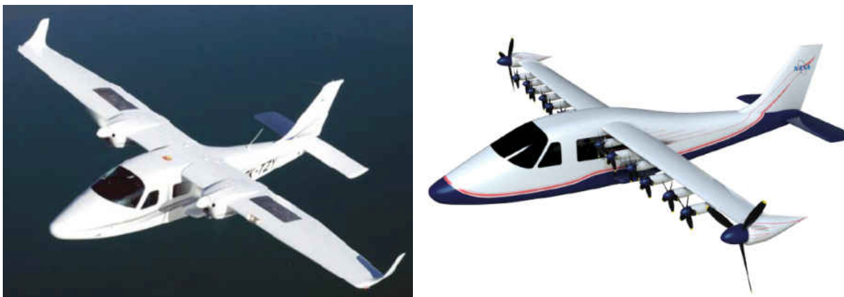
Figure 4. Tecnam P2006T aircraft and SCEPTOR design (Dubois et al., 2016; Moore et al., 2014)
