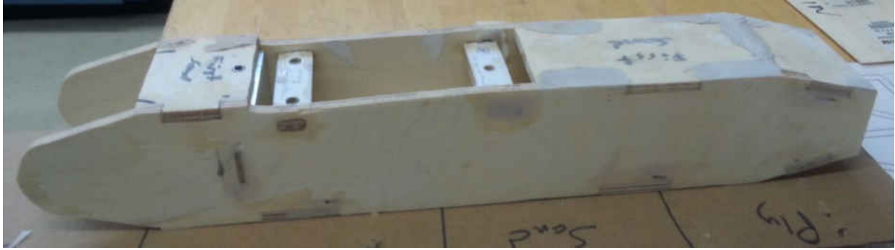
Figure 23. Fuselage and aluminum bulkhead before nose covering and sanding process
