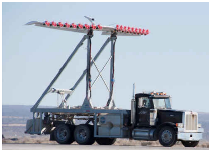
Figure 3. LEAPTech experimental testbed (Stoll, 2015)
