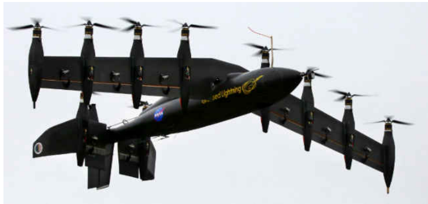
Figure 7. GL-10 50% scale aircraft with 10.5 ft wingspan (Rothhaar et al., 2014)
