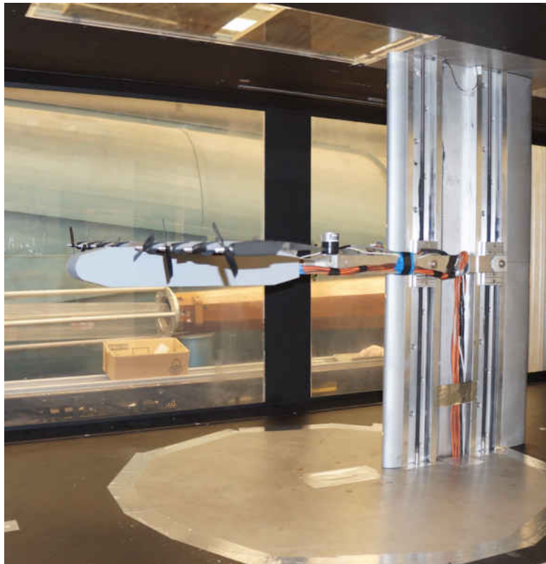
Figure 26. Model and support system in test section
