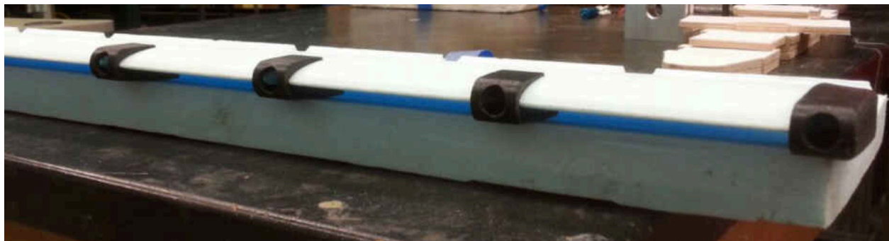
Figure 21. Motor mountings along the leading edge
