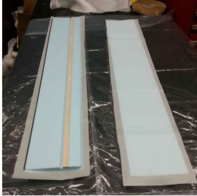
Figure 18. Blue foam wing core, strut, rod and fiberglass
