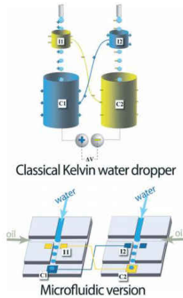
Fig. 25. Schematic of the microfluidic Kelvin water dropper[42].
