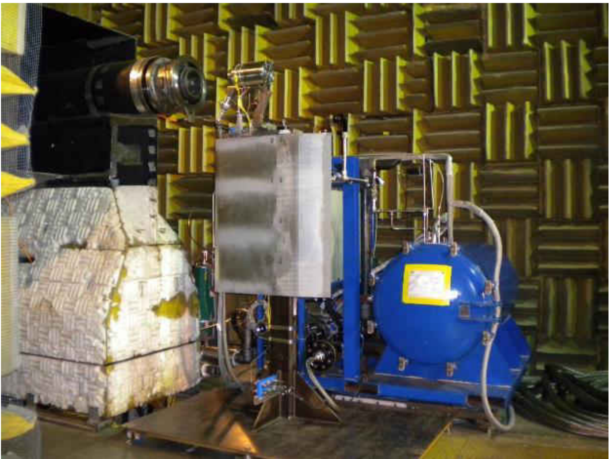
Figure 28 Initial testing Configuration of CJES Combustor in the Jet Noise Laboratory. (12)
