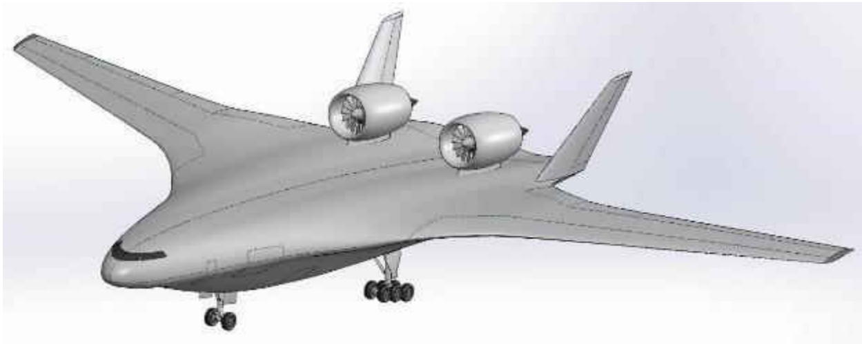
Figure 11. Boeing Concept of the Hybrid Wing Body Aircraft. (5)
