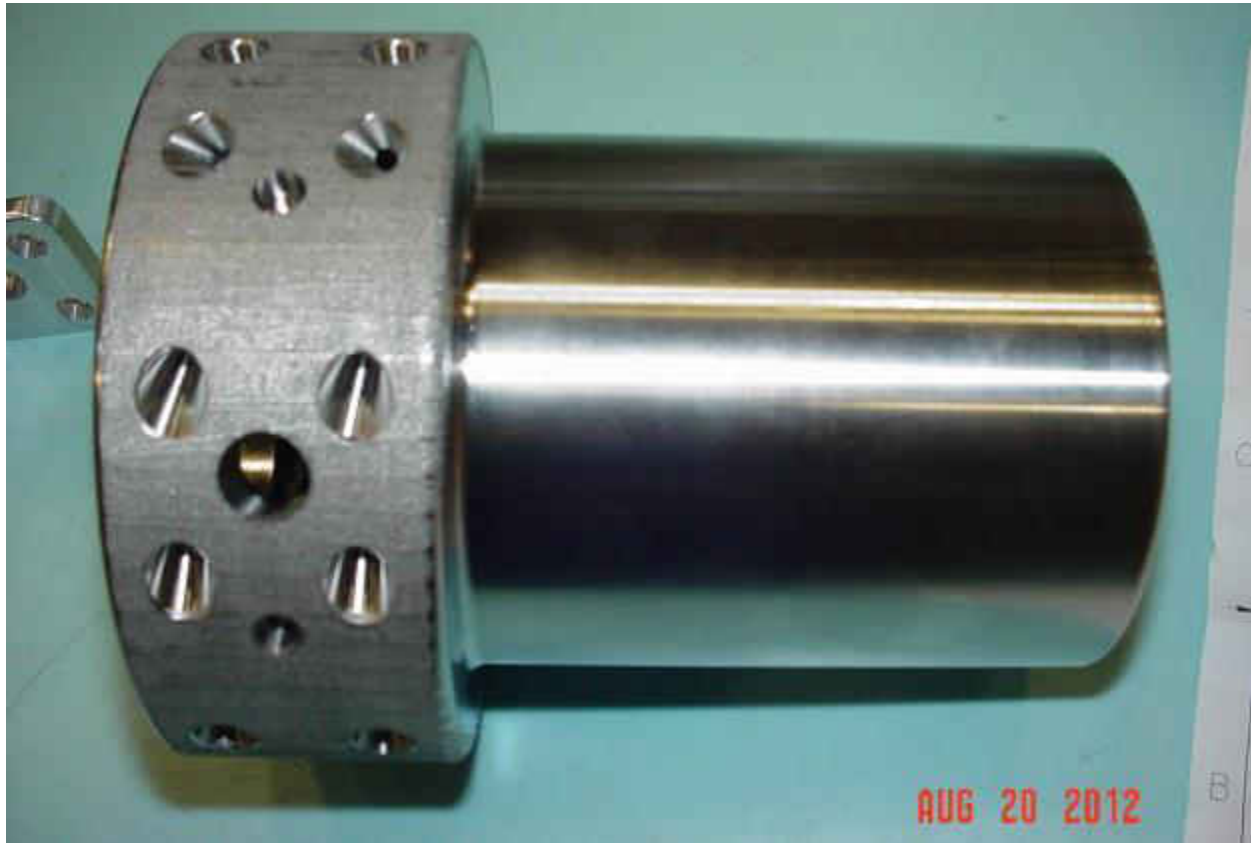
Figure 26 Finished CoCr Combustor Liner. (12)
