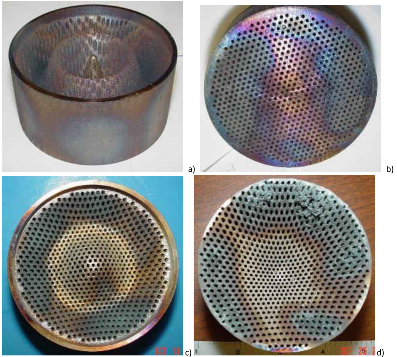
Figure 50 Core Flow Conditioners Exhibiting Nonuniform Heating. Pictures a) and b) show upstream and downstream view of the same part, c) shows a Single Sinusoid, d) shows a Concave Unit. (12)
