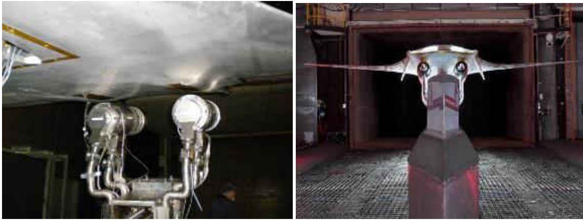
Figure 43 Hybrid Wing Body Model in 14x22' Tunnel with the CJES Units and Model Support. (12)
