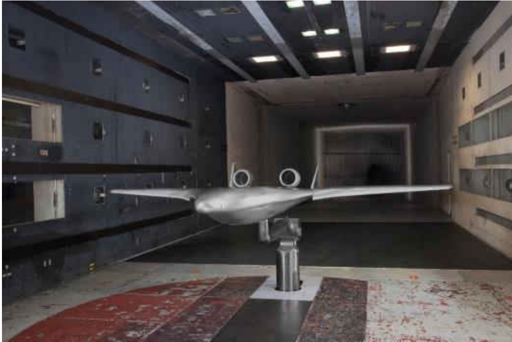
Figure A-5 Aerodynamic Test of the HWB in the 14x22' Subsonic Wind Tunnel. (40)
