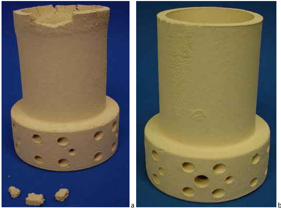
Figure 20 Failed Ceramic Combustor Liners, a) New Coarse Material, and b) New Fine Material. (12)
