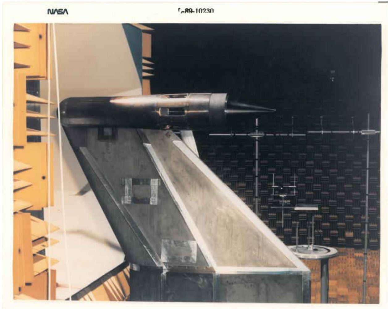
Figure 4 Boeing Nozzle Test Rig in 1989, (NASA photo L-89-10230)
