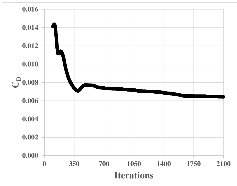
Figure 4.7 Convergence of C_D with the Transition \kappa - \omega SST Model for the G1 Profile.
