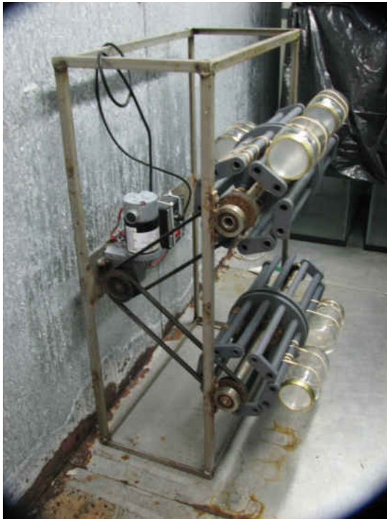
Figure 4.1. The plankton wheels used in an experiment designed to test the effect of water movement on oviposition in Lirularia succincta .
