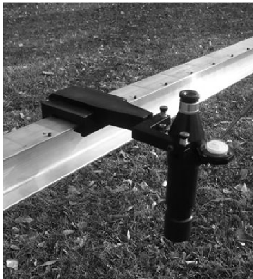
Figure 2.2. Photograph of optical point sampling device and sampling bar. Photo W. Keammerer.
