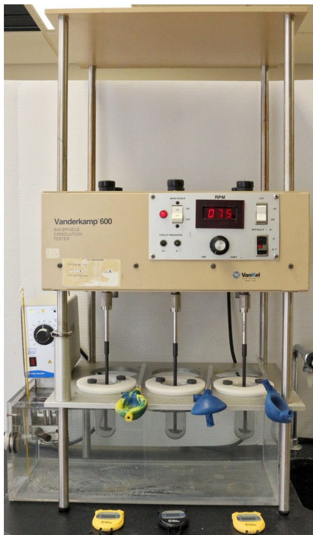
Figure 9.4 Dissolution Apparatus 2 with small-volume vessels [12]
