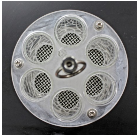
Figure 7.4 Disintegration Test Basket-Rack Assembly [11]
