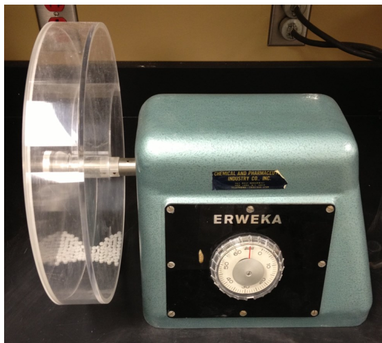
Figure 7.2 Erweka Tablet Friability Apparatus [7]
