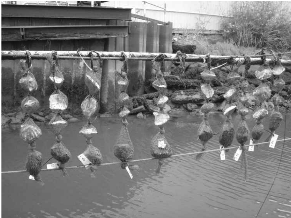
Figure 3. Experimental set up shown before deployment: 20 mesh bags hung 15 cm apart from a 2.5 m long PVC pipe. Each mesh bag has three shells of the same substratum type with knots between each to maintain spacing. A rock is tied at the bottom of each bag for weight
