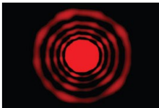
Figure 5-3 (b) Diffraction pattern a small particle[23]
