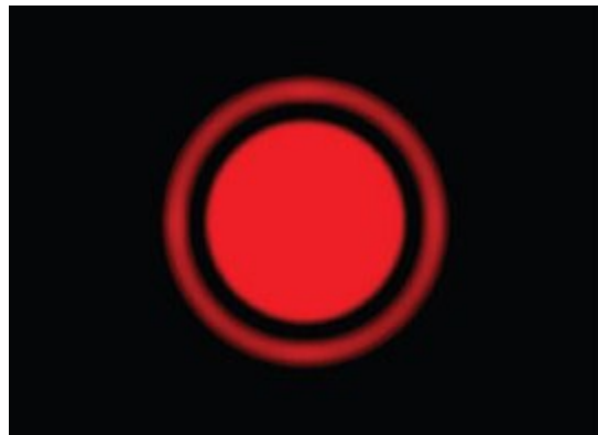
Figure 5-3 (a) Diffraction pattern of a large particle
