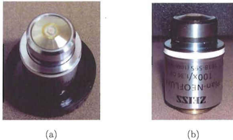
FIGURE 3.8: Top view (a), and side view (b) of a glued micro-concave mirror substrate on top of a Zeiss microscope objective ( NA = 1.3 ).
