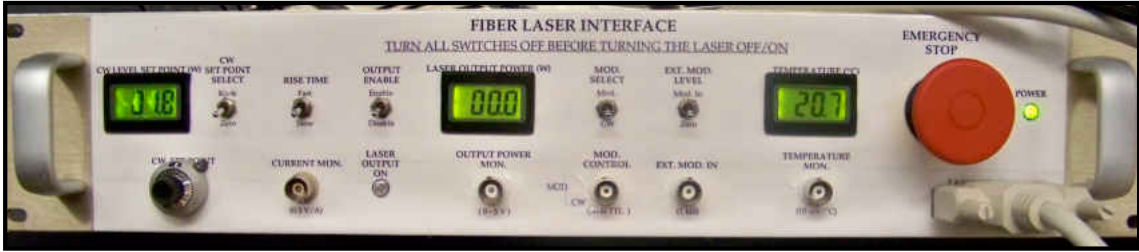
Figure 2.24. Picture of the home-built, fiber-laser control box, including several LCD displays showing the manual CW set-point, power output and laser temperature, and the emergency stop button.
