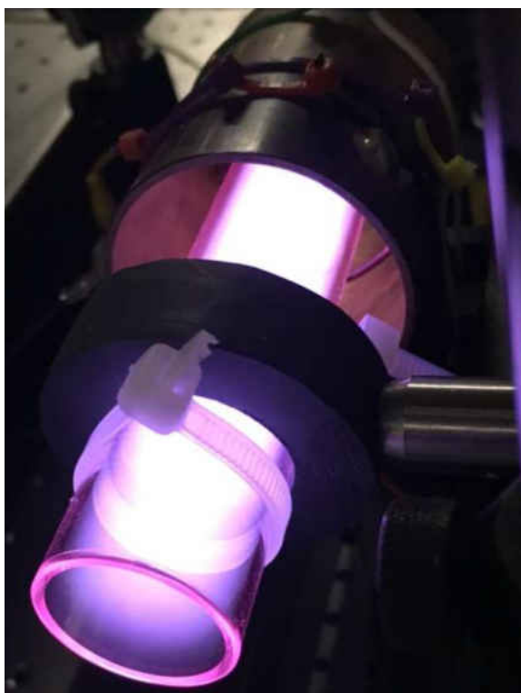
FIG. 14: A photograph of a Kr cell with an RF discharge inside. This specific cell was used to provide a reference to lock to the 819 nm transition.
