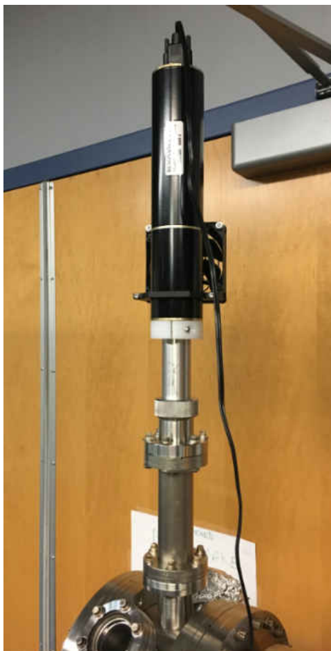
FIG. 28: A photograph of the UV lamp, as seen mounted into the vacuum chamber. The plasma forms near the center of the chamber.
