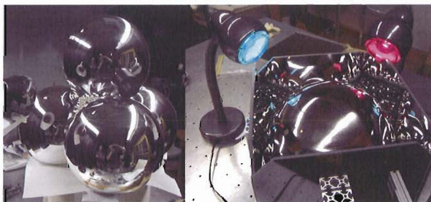
Figure 1.13. Photograph of the stacked sphere configuration (left) and the Sinai cube apparatus (right).
