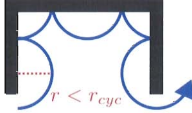
Figure 2.14. Schematic of the skipping orbit regime which occurs when r > r_{cyc} . Where r_{cyc} is defined as the radius of an inscribed circle that will just fit inside a billiard
