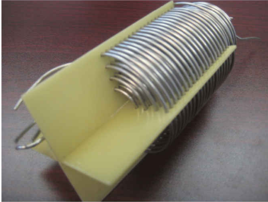
FIG. 12: The high power heater before installation
