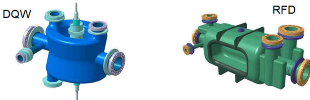
FIG. 20: Crab cavity concepts for the HL-LHC upgrade, DQW and RFD cavities for vertical and horizontal bunch crabbing.
