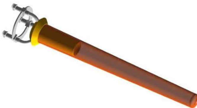
FIG. 23. A diagram of g11 cryotarget with L=40\text{cm} and R=2\text{cm} .
