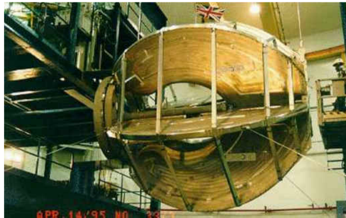
FIG. 21. The coils of the CLAS toroidal magnet prior to installation of the rest of the detector. Image Source [27]
