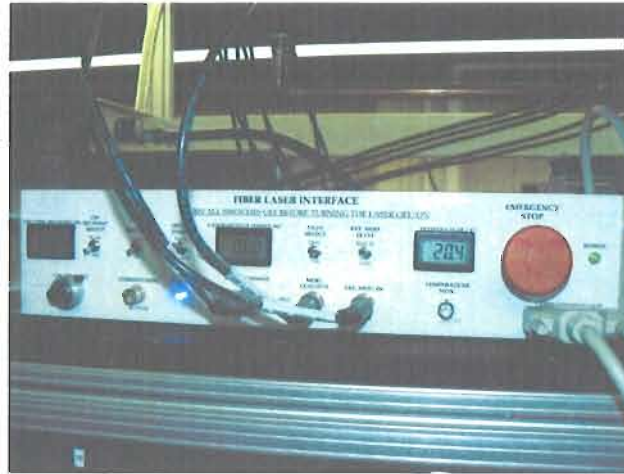
FIGURE 3.25: The fiber laser control box, which controls the fiber laser and acts as a modulation interface.
