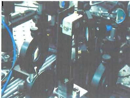
FIGURE 3.23: The mechanical shutter used for the pyramid MOT laser. It is mounted near the focus of a telescope system.
