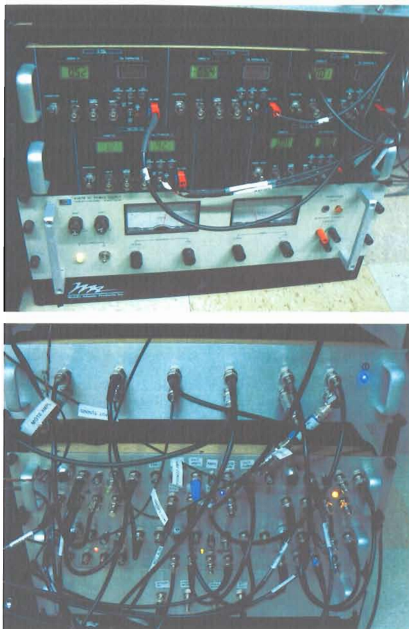
FIGURE 3.3: The electronics racks. The top image shows the racks holding some of the magnetic coil electronics. The bottom image shows the electronics for the AOMs used in our experiment.
