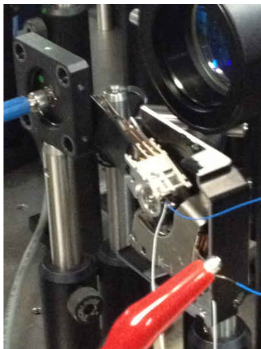
FIG. 51: A homemade shutter created with a hard-drive motor. A piece of metal is epoxied to the fins to serve as the light block and is placed directly in front of a multimode fiber used to direct fluorescence to the photocathode of a PMT.
