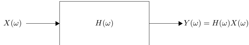
FIG. 64: Demonstration of the linear response of a filter network. The sample can be thought of as a filter with response function H(\omega) . In the diagram, X(\omega) is synonymous with the incident field and Y(\omega) with the transmitted field.
