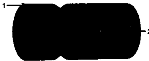
FIG. 39: Cavity with no rounding at (1) the outer conductor edges and (2) the spoke base.
