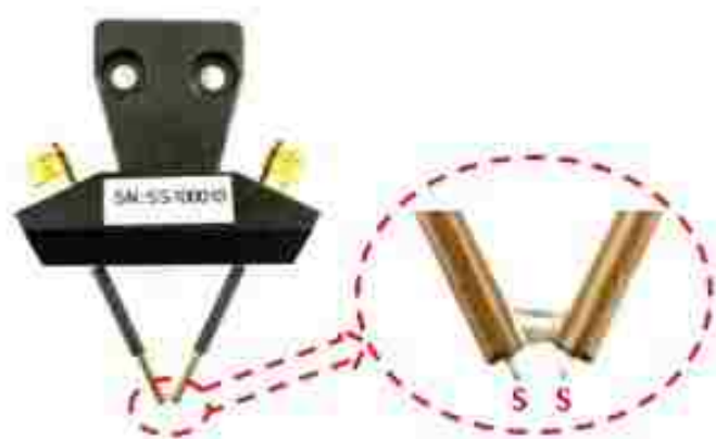
Figure 3.1. 1mm pitch D-probe with a detailed view of tips.
