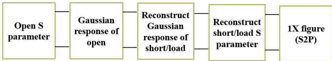
Figure 2.3. Workflow of the 1X-Reflect SFD method.
