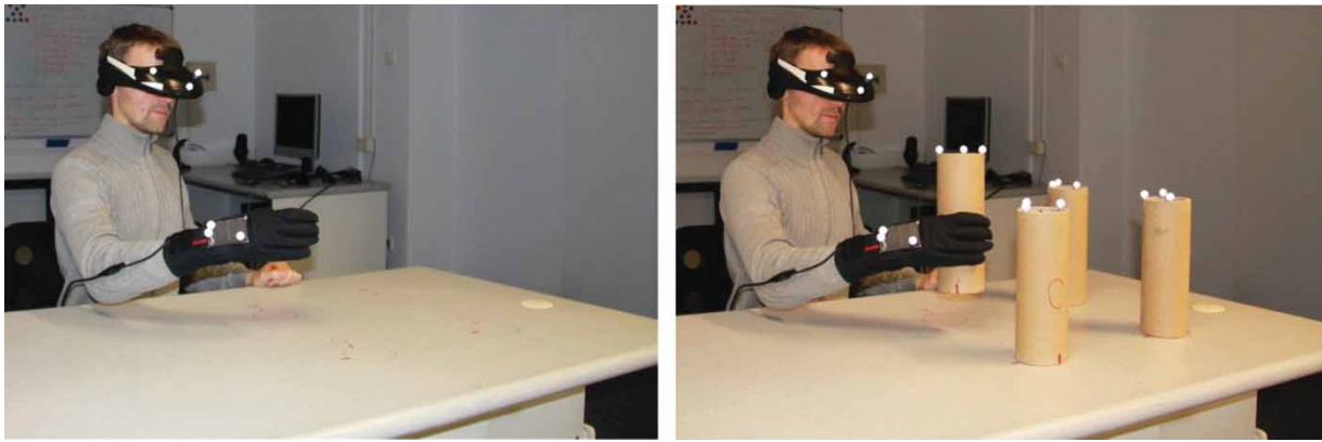
Figure 2. The workstation presenting a simulated work performed without real objects (left side) and with real objects (right side) (Photo: Grabowski A.)
