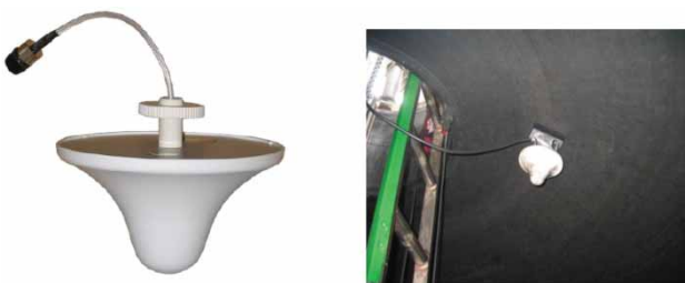
Figure 5. The cone-shaped directional antenna and its place in an residuum desulfurization (RDS) reactor.
