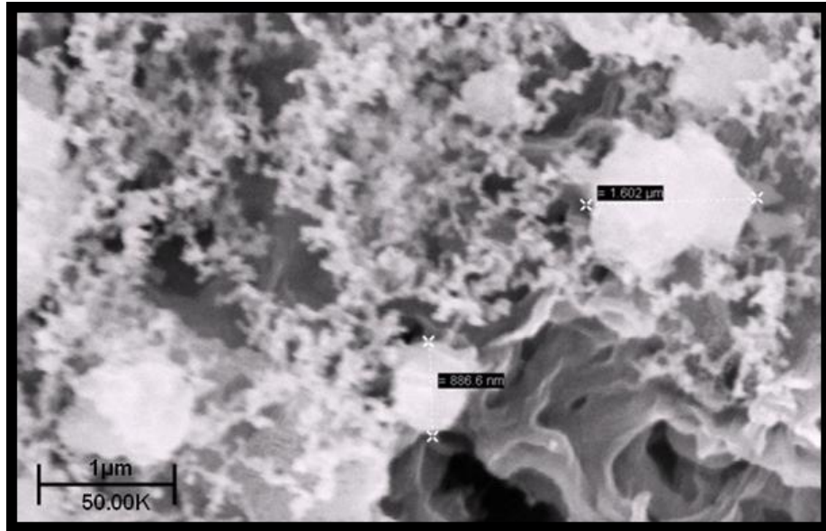
Figure 6.38 b) High magnification scanning electron micrograph of 1 \times 10^7 cfu/ml E. coli exposed to MIC NP101 for 6 hours
