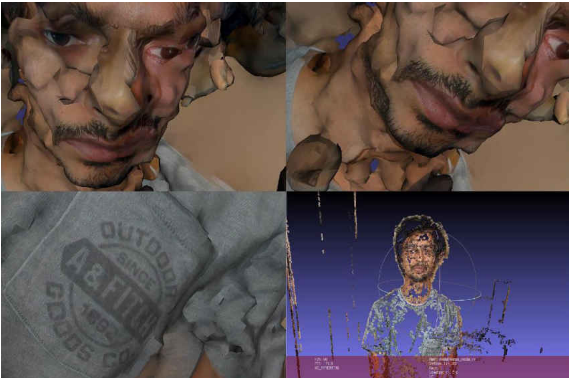
Figure 48 Low Detail 3D Model Reconstruction of Human Face with 30 Images
