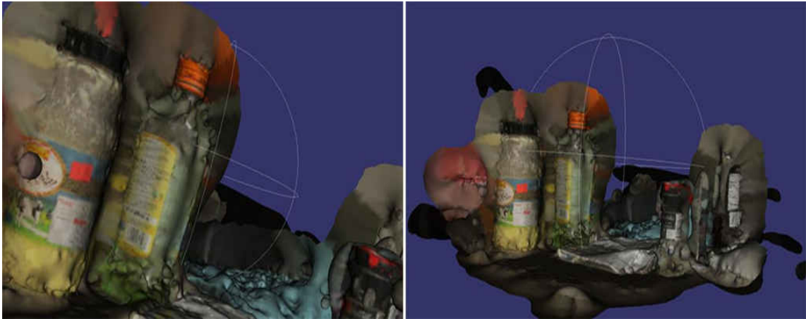
Figure 47 Low Detail 3D Model Reconstruction of Objects From 3 Images
