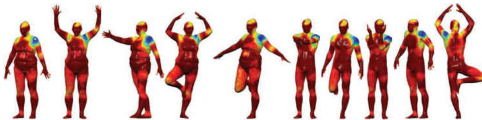
Figure 2.6: The Euclidean distance between the descriptor of the white point on the left shoulder obtained in [7] and those of the other points are represented. Red color corresponds to the higher distances. As it is observed, the point is detected locally with high level of sensitivity and specificity. The figure is taken from [7].
