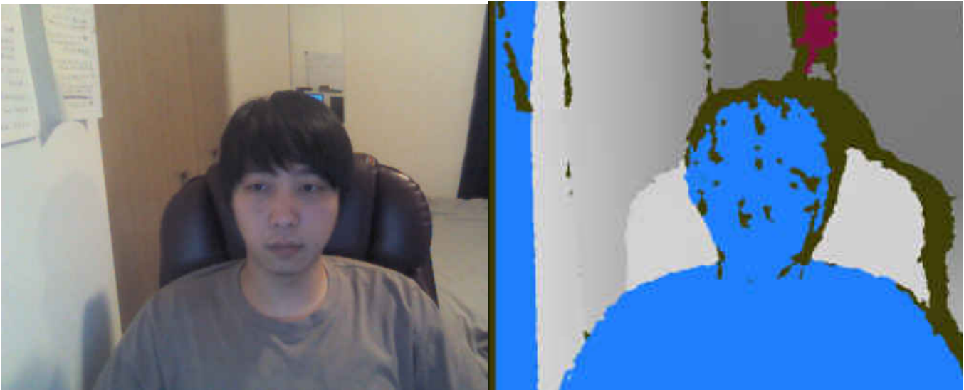
Figure 2.4 An example of a color frame and a depth frame
