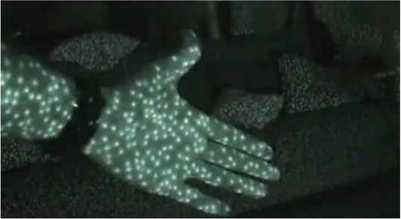
Figure 2.3 Infra-Red dots projected on the scene[27]
