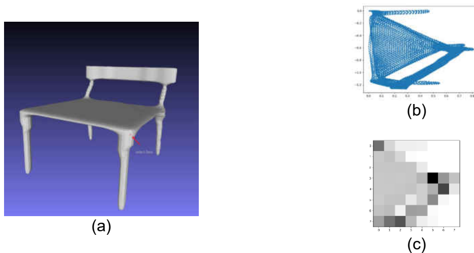
Figure 24 Example of a spin image (a) a face select on a mesh of chair, (b) the distribution of all other vertices in (\alpha, \beta) coordinates, (c) the spin image with 8 uniform bins on both axis.
