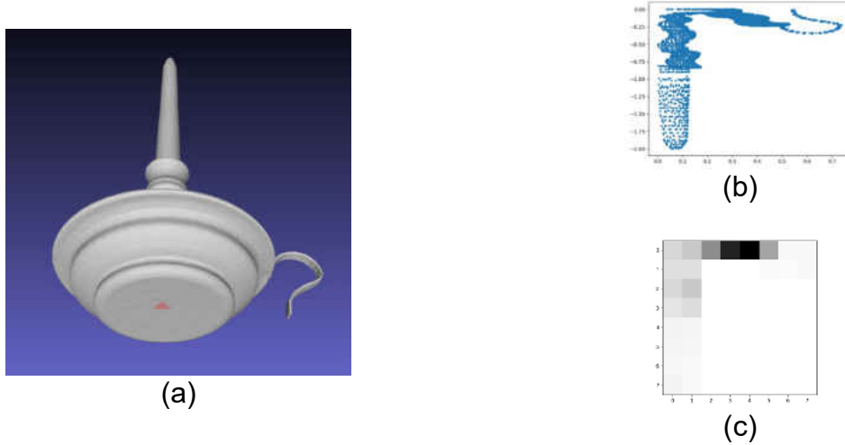
Figure 25 Example of a spin image (a) a face select on a mesh of candelabra, (b) the distribution of all other vertices in (\alpha, \beta) coordinates, (c) the spin image with 8 uniform bins on both axis.
