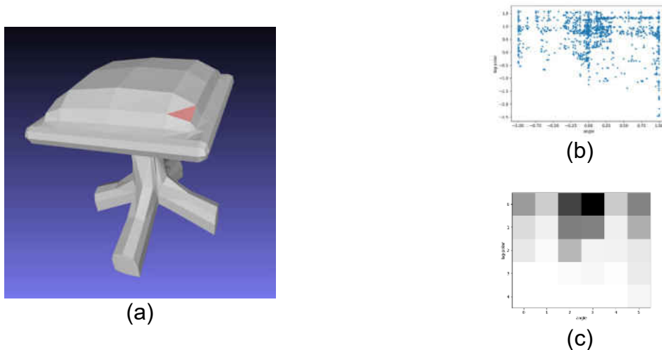
Figure 17 Example of a shape context (a) face select on a mesh of chair, (b) the distribution of all other vertices in \log(r) and angle space, (c) the shape context with 5 \log(r) bins and 6 angle bins.
