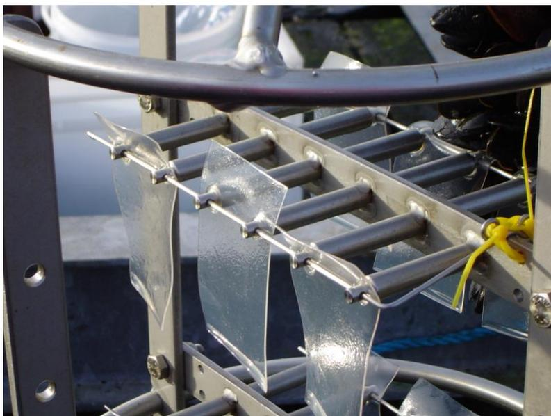
Figure 1-7 Silicone rubber passive sampling sheets mounted on a sampler frame
