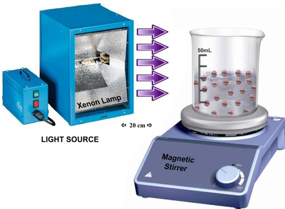
**Fig.4.4.** Standard experimental design using a Xenon lamp with unidirectional irradiation of the reaction vessel (50 ml glass beaker) containing aqueous suspension of TiO<sub>2</sub> in the presence of test sample.
