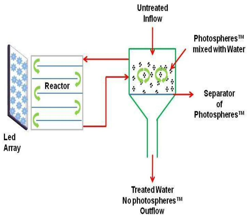
**Fig.4.19.** Schematic diagram of potential pilot system for water treatment
