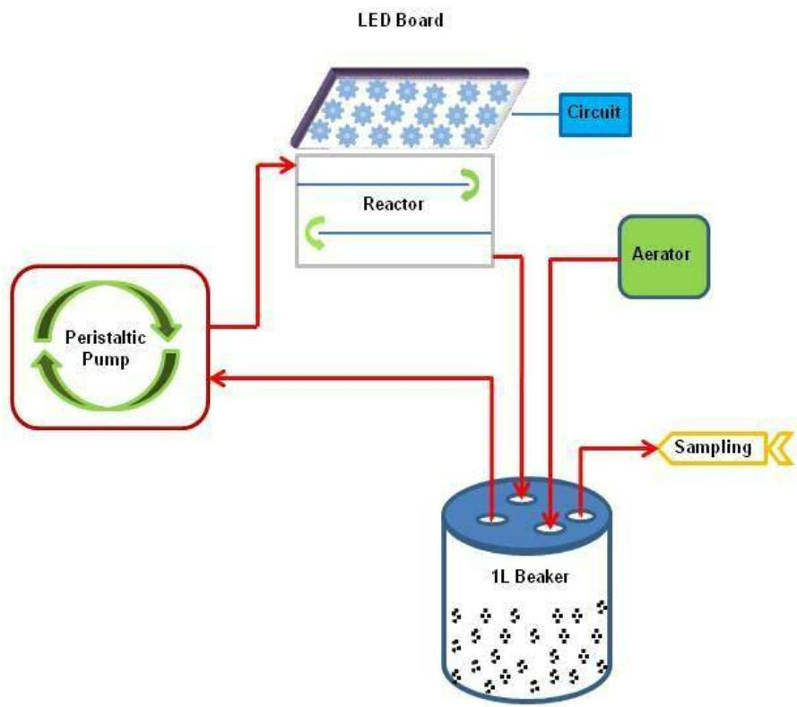
**Fig.4.6.** Schematic representation of novel LED photo reactor
