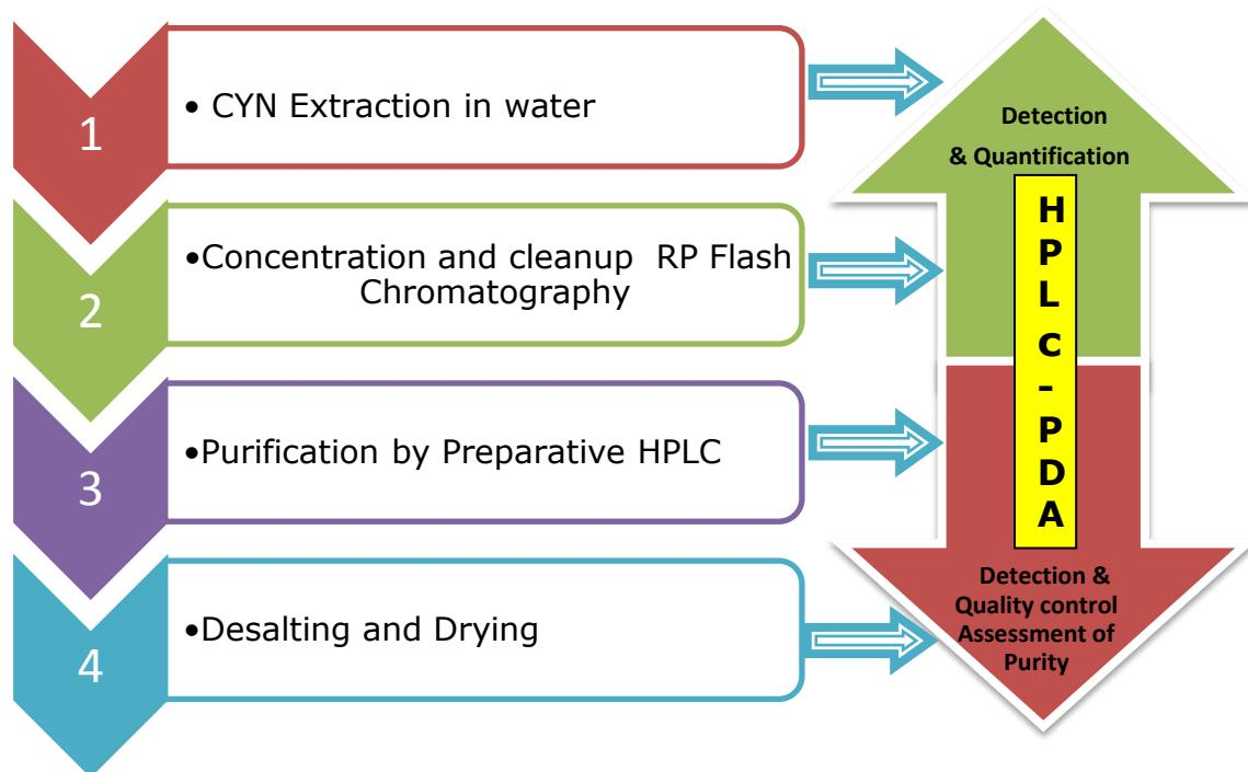
**Fig. 2.2.** Schematic diagram of the HPLC based purification of cyanotoxins (Edwards *et al.*, 1996).
