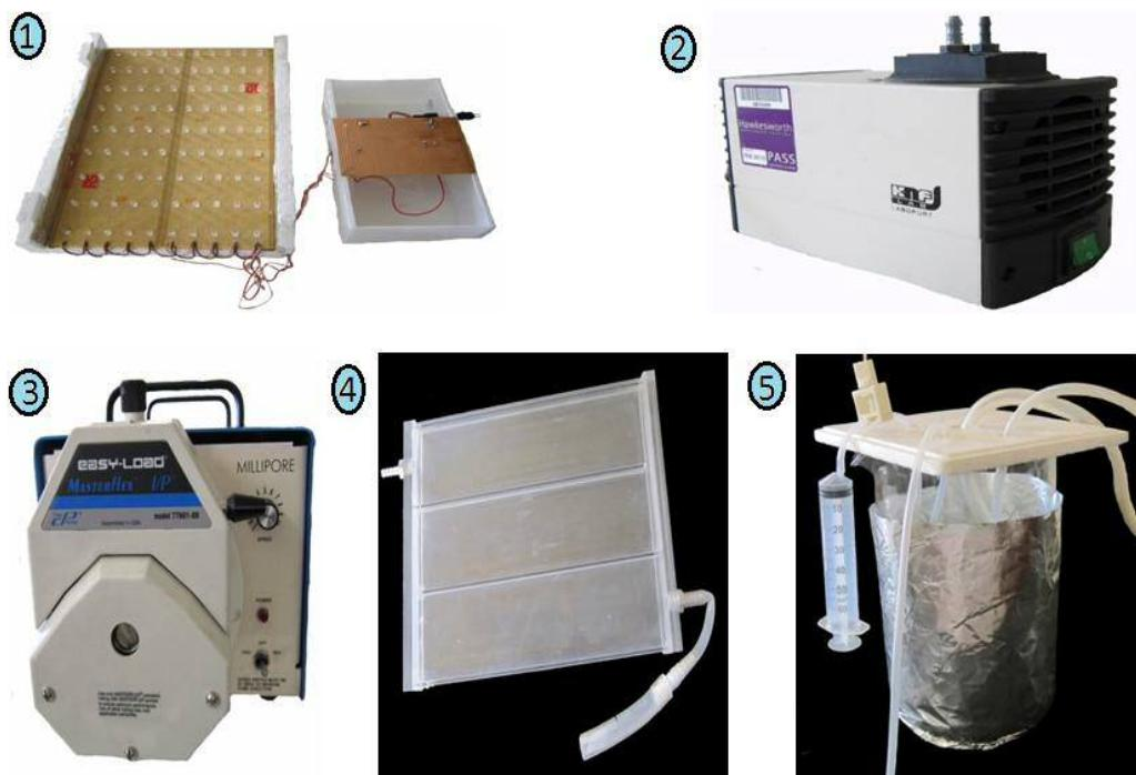
**Fig.4.7.** Photographs represents the parts of the novel LED reactor **(1)**. UV LEDs arranged on PCB and connected with circuit board. **(2)**. Aerator. **(3)**. Peristaltic pump. **(4)**. Reaction container. **(5)**. 5 L glass beaker closed on top. Tubing in the beaker for sample intake and outtake, sampling (with syringe) and sparging (aerator).
